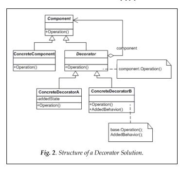
Figure 2 [6] shows the general structure of a solution with the Decorator design pattern, which presents different components and relationships. Table I describes the components of Figure 2.
