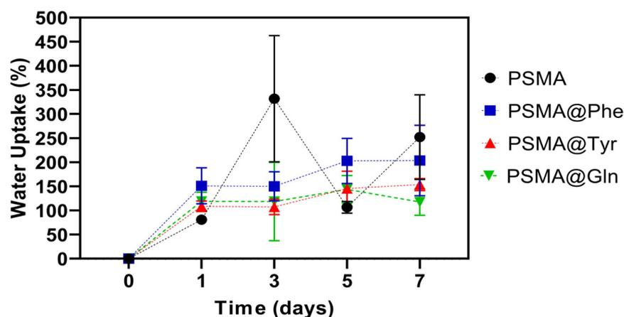
Figure 9. Water absorption capacity of PSMA and PSMAf over time.
