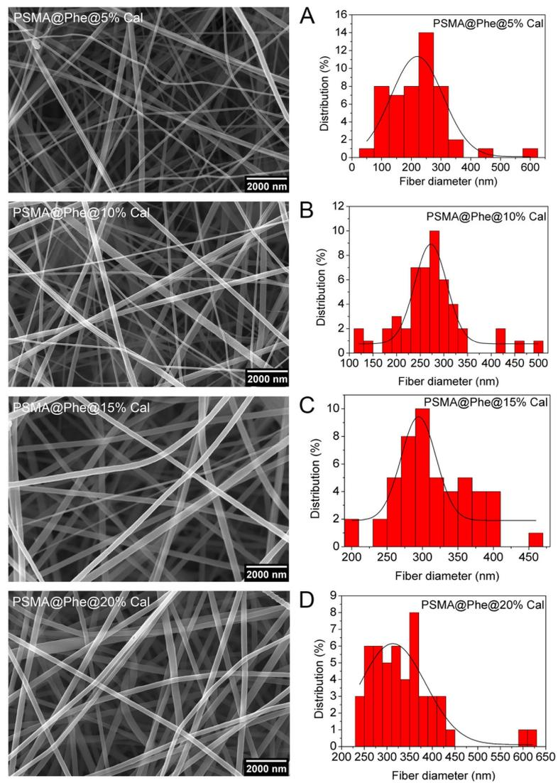
**Figure 6.** SEM images PSMA@Phe with different concentrations of *C. officinalis*, (A) 5.0, (B) 10, (C) 15 and (D) 20 wt.%. Magnification 30,000 $\times$ .
