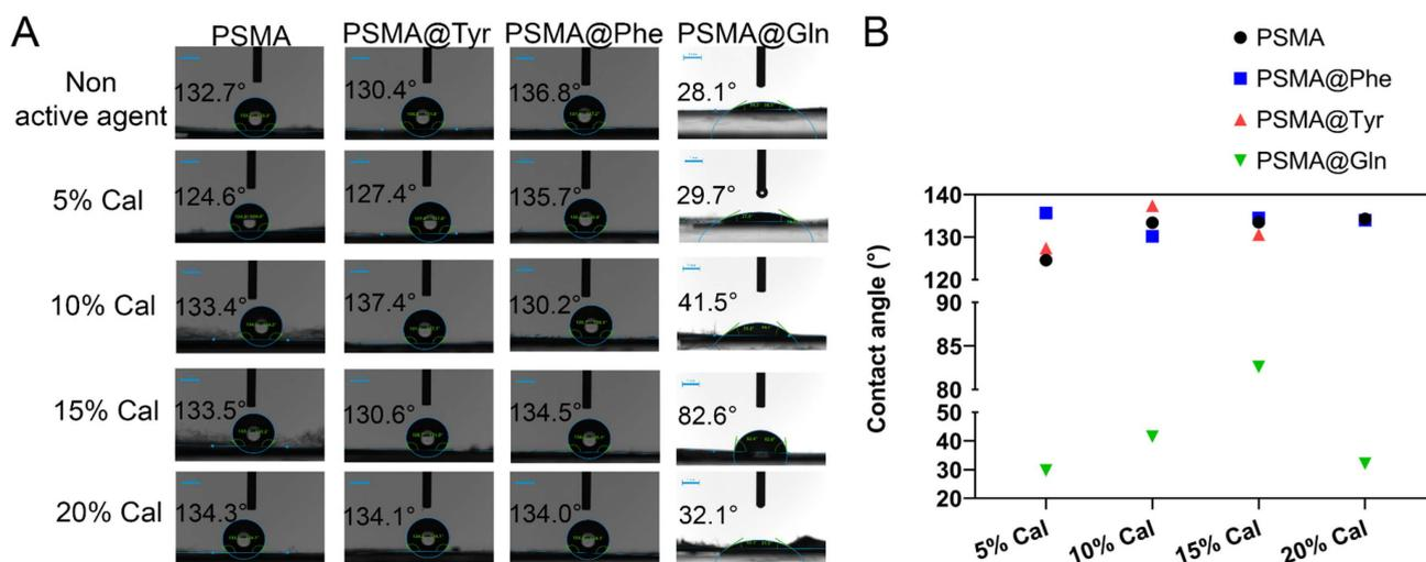
**Figure 8.** (A) Contact angles of PSMA and PSMAf in the absence and presence of 5, 10, 15 and 20 wt.% of *C. officinalis* (scale bar: 1 mm), (B) Graph of the contact angles of PSMA and PSMAf.
