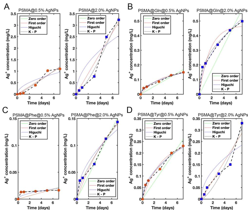
**Figure 10.**  $\text{Ag}^+$  release curves from mats containing 0.5 wt.% (red circle) and 2.0 wt.% (blue square) concentrations of AgNPs: (A) PSMA, (B) PSMA@Gln, (C) PSMA@Phe and (D) PSMA@Tyr.
