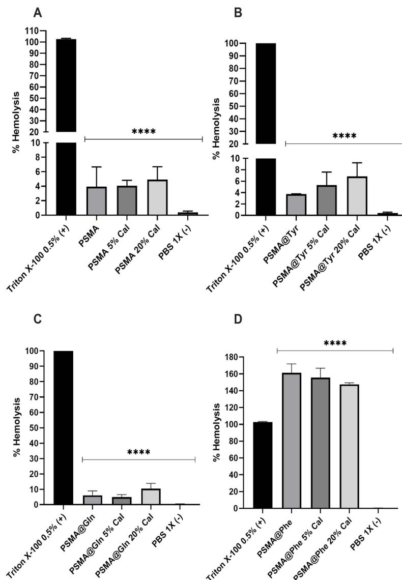
**Figure 14.** Percent hemolysis of polymeric mats (PSMA and PSMAf) with different concentrations of active agents. (A) PSMA, (B) PSMA@Gln, (C) PSMA@Tyr and (D) PSMA@Phe. Data were analyzed using Dunnett's multiple comparisons test; \*\*\*\*  $p < 0.0001$  compared to the positive control group (Triton X-100).
