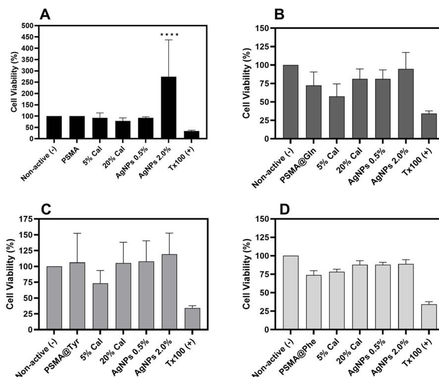
**Figure 13.** Percentage cell viability of NIH/3T3 fibroblasts versus PSMA and PSMAf mats with different concentrations of active agents. (A) PSMA, (B) PSMA@Gln, (C) PSMA@Tyr and (D) PSMA@Phe. Data were analyzed using Dunnett's multiple comparisons test; \*\*\*\*  $p < 0.0001$  compared to non-active.
