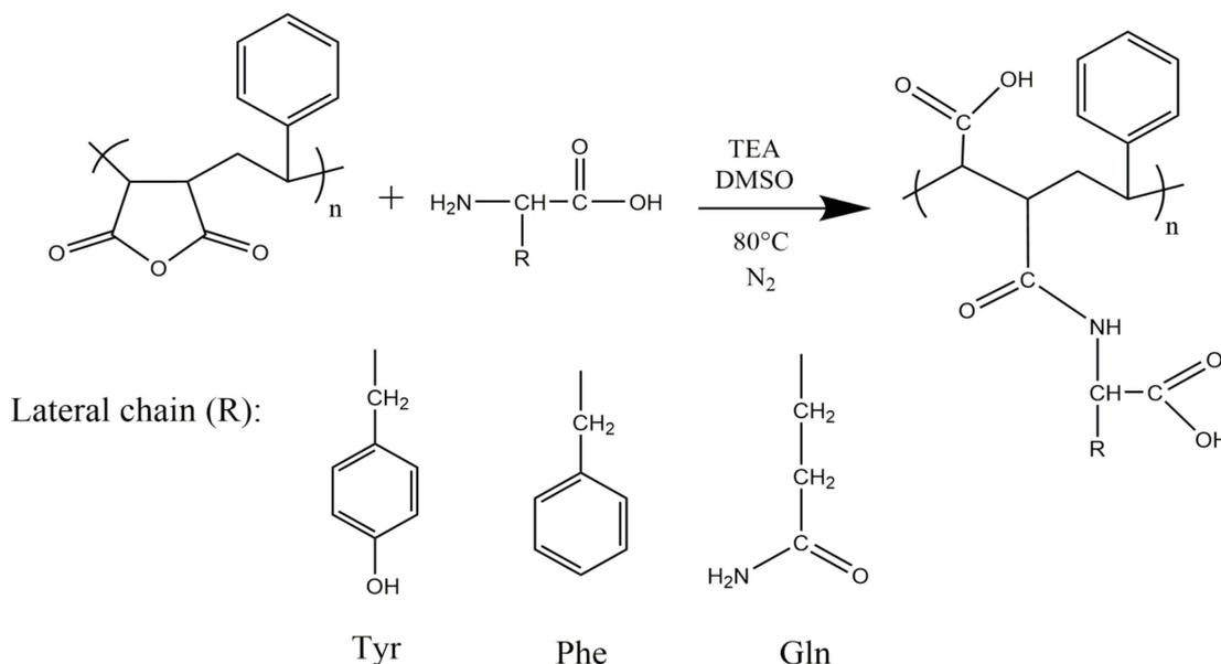
**Figure 1.** Schematic of the functionalization reaction of PSMA with different amino acids.
