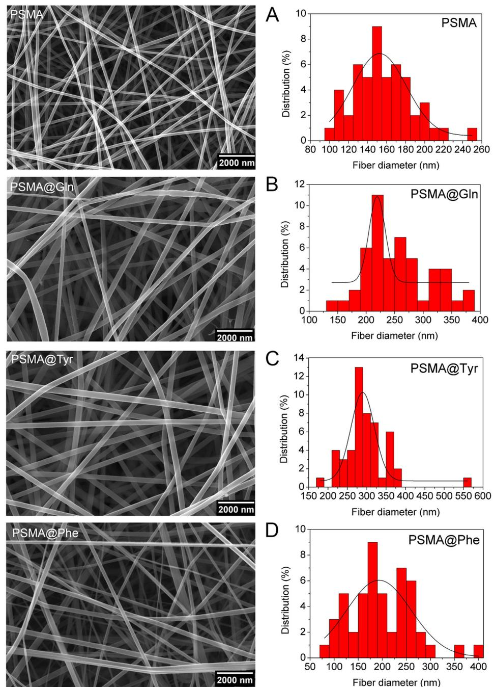
**Figure 3.** SEM images of mats of (A) PSMA, (B) PSMA@Gln, (C) PSMA@Tyr and (D) PSMA@Phe. Magnification 30,000 $\times$ .
