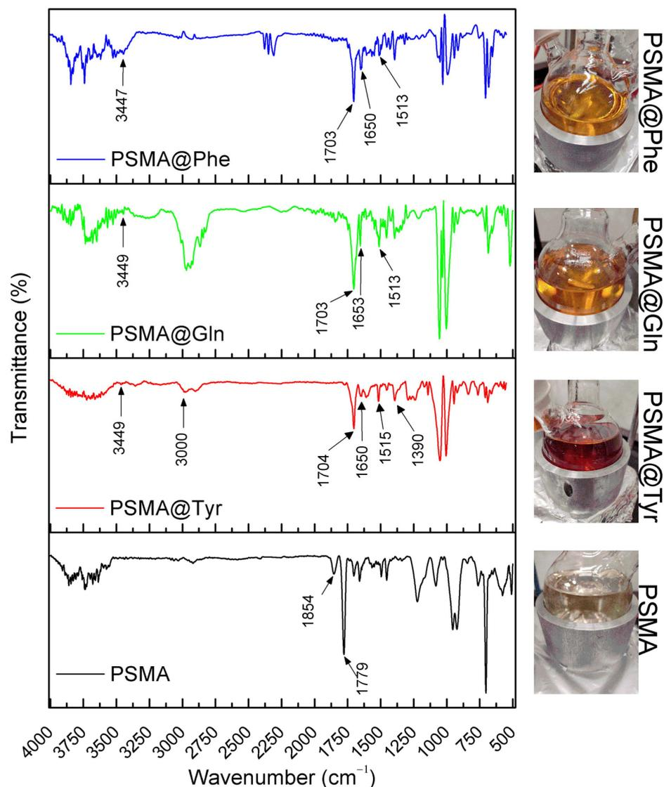
**Figure 2.** ATR-FTIR spectra of mats of PSMA and PSMAf.
