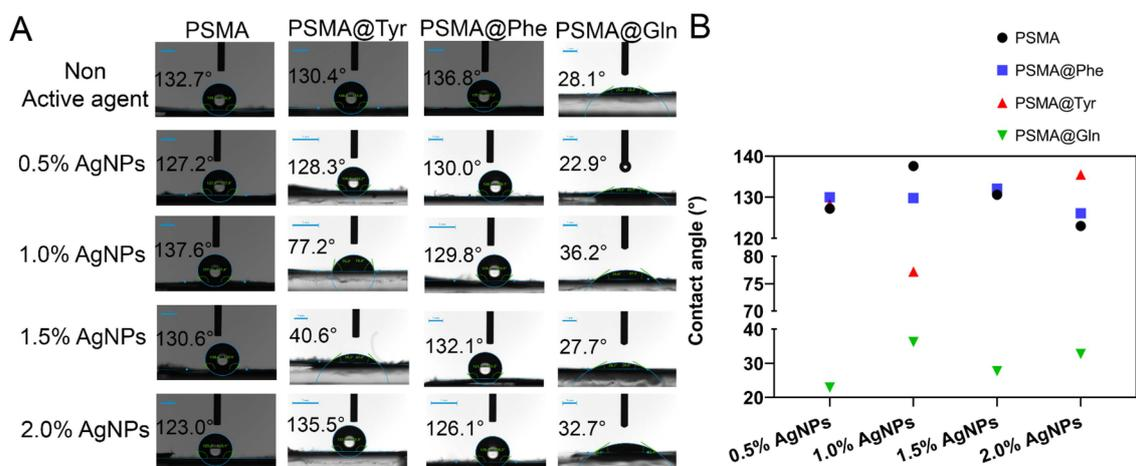
**Figure 7.** (A) Contact angles of PSMA and PSMAf in the absence and presence of 0.5, 1.0, 1.5 and 2.0 wt.% AgNPs (scale bar: 1 mm), (B) Plot of the contact angles of PSMA and PSMAf.
