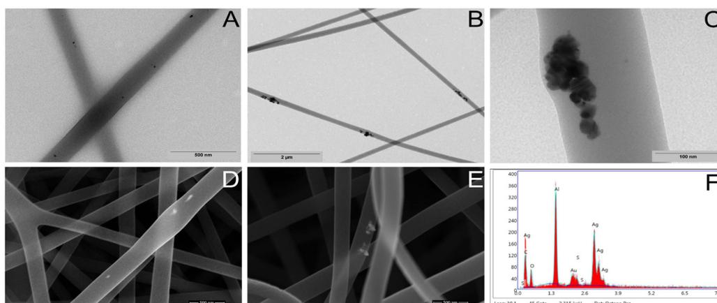
**Figure 5.** (A) TEM image of PSMA@Phe fibers containing 0.5 wt.% AgNPs, (B) TEM image of PSMA@Phe fibers containing 2.0 wt.% AgNPs, (C) 100,000 $\times$  magnification image of PSMA@Phe containing 2.0 wt.% AgNPs, (D) FESEM image of PSMA@Phe mats containing 1.0 wt.% AgNPs, (E) FESEM image of PSMA@Phe mats containing 1.5 wt.% AgNPs and (F) X-ray energy dispersive spectrum (EDS) of image (E).
