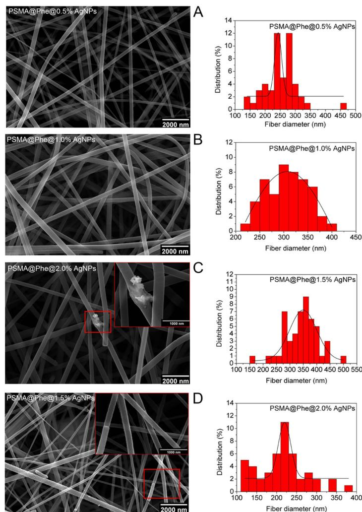
**Figure 4.** SEM images PSMA@Phe with different concentrations of AgNPs, (A) 0.5, (B) 1.0, (C) 1.5 and (D) 2.0 wt.% Inset in image (C) and (D) corresponds to higher magnification area. Magnification 30,000 $\times$ .
