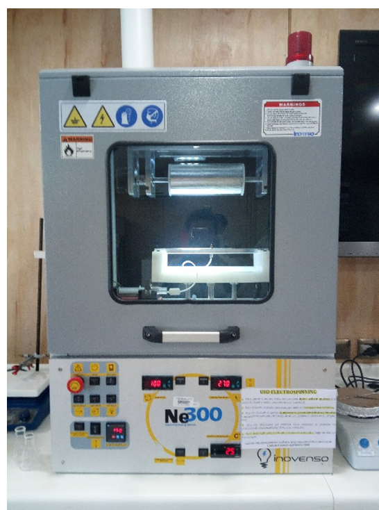
Fig. 2. Electrospinning equipment with rotating cylindrical collector.
